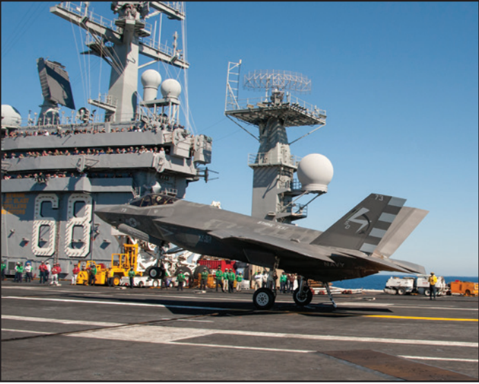
An F-35C Lightning II pictured catching a wire on board Nimitz during the Joint Strike Fighter’s first carrier suitability flights in 2014.
