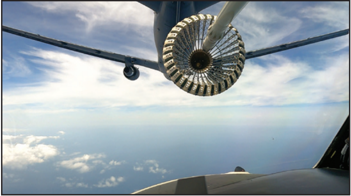
VAW-124 Bear Aces E-2D Advanced Hawkeyes conduct air-to-air refueling from a U.S. Air Force KC-46 Pegasus, a first for a fleet airborne command and control squadron.
