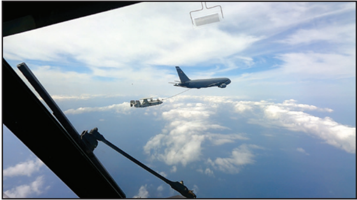
VAW-124 Bear Aces E-2D Advanced Hawkeyes conduct air-to-air refueling from a U.S. Air Force KC-46 Pegasus, a first for a fleet airborne command and control squadron.
